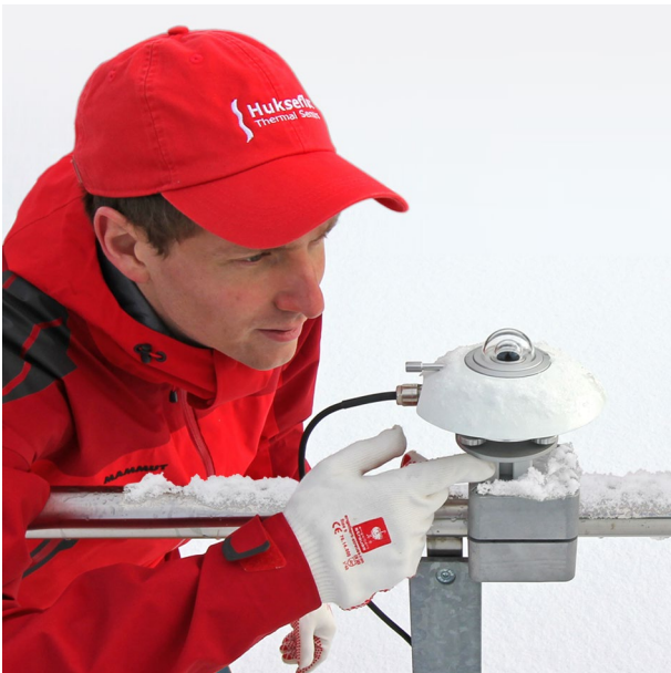
Figure 4 SR25 accelerating sublimation of snow, here shortly after snowfall.
