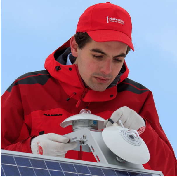
Figure 4 SR20-D2 Class A pyranometers with digital output for GHI (Global Horizontal Irradiance) and POA (Plane of Array) measurements.
